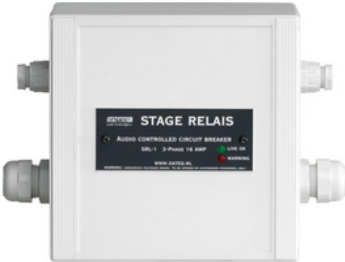
**Relay box**, for SPL-3, SPL3-TS, SPL-5, SPL-6 and SPL-D2 The SRL-1 is build as relay extension box for the SPL3, SPL3TS, SPL5 and SPL6 limiters and the SPL-D2 display. Linked to one of the SPL series limiters or display, the SRL-1 allows a warning light and power cut out on exceeding the pre-set sound level. Linked to the SPL-D2, the software allows a sanction threshold, delay and duration set point.
