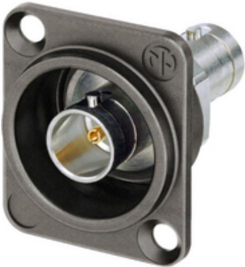
NEUTRIK UHD BNC panel jacks provide low return loss values at high frequencies, which typically occur in high-definition video signal transmissions. The machined brass body ensures a rugged and non-abrasive connection. Due to being recessed in the D series body (audio industry standard) they are additionally protected.
