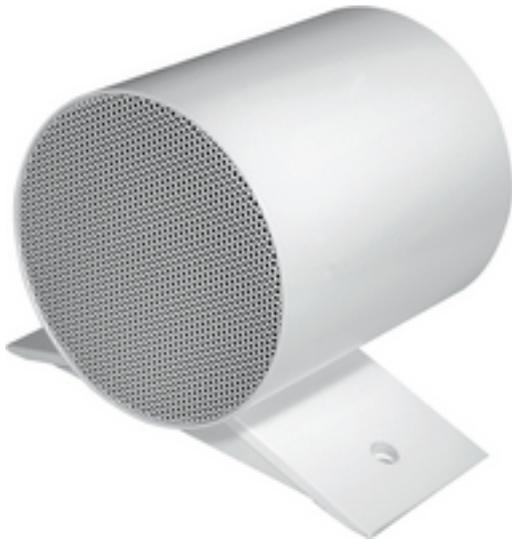
The sound projector with a power capacity of 10 W is fitted with two 13 cm full range speakers and a 100 V transformer with 4 power taps. A robust plastic-coated aluminium housing in RAL9010 and a vandal-resistant aluminium mounting plate ensure a permanent installation of this speaker. The 2-pole ceramic terminal and thermal fuse as well as the waterproof speaker ensure extra operating reliability.
