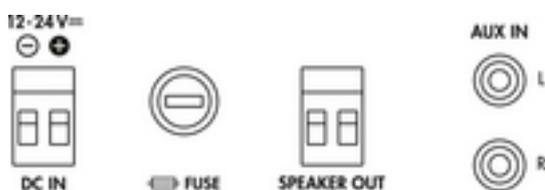
The MMA-130 is a mono class D mixing amplifier with 30 W (8 Ohm). The device has been developed in-house according to the specifications of a globally operating crane manufacturer and thus is perfectly matched to the application in the crane operator's cabin. The MMA-130 is used for the crane operator's announcements made to people within the pivoting range of the crane.
