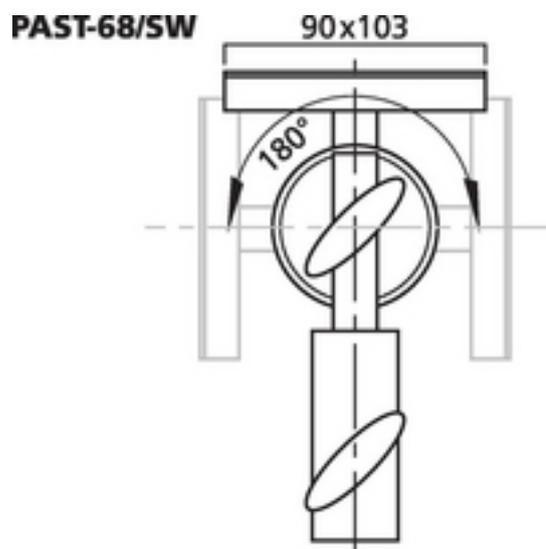
Push-on tilting adapter with mounting plate
